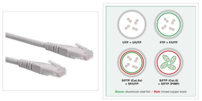
Patch cable for networking connections between devices. Prepared unshielded Twisted Pair cable with RJ-45 connectors on both ends. Durable due to moulded kink protection. Flexible cable, suitable for narrow bending. High quality plugs with gold plated contacts. Contact settings 1:1, in accordance with the EIA/TIA 568 standard. Construction: 4-pair stranded copper wire.
