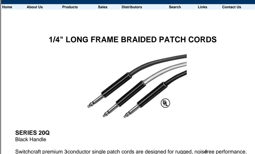
Nickel-plated plugs eliminate the need for periodical cleaning which keeps your audio signals clear. Color cords provide instant visual identification with a choice of three lengths. All cables are fully shielded with rugged, braided thermoplastic outer jackets. Plug handles are black. Audio patch cords are available with other lengths and brass plugs, if desired. Contact Switchcraft for specifying assistance and cable length tolerances.
