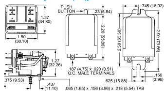
Note: The 263/268 Series Relay is a 15 Amp Version of the 262/267 Series Relay Except With .187" Quick Connect Terminals. The User May Utilize the 260 Series Dimensions on Page 15 for Further Detail.
