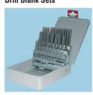
Manufactured from High Speed Steel. Finished ground to h8 tolerance. Sets 1-6mm: 51 pieces in 0.1mm steps. Sets 6-10mm: 41 pieces in 0.1mm steps. Supplied in metal indexing box.
