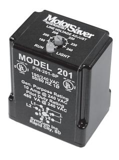
The Model 201-xxx-SP is an 8-pin octal base plug-in voltage monitor designed to protect single-phase motors regardless of size. It can be used on 95-120VAC (201-100-SP) or 190-240VAC (201-200-SP) motors to prevent damage caused by low voltage. High voltage detection is included on the 201-200-SP-T-9 model.
