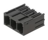
Single-row, high-performance male connector, for side-byside mounting without losing any poles or with patented flange for fast fixing without tools. Maximum connection and operating reliability thanks to pin arrangement that prevents wrong connections, unique coding diversity and additional fixing in flange. 3.5 mm pin length is optimised for wave soldering, plug-in direction 270° to solder pins.
