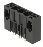
Single-row, high-current male connector, for side-byside mounting without losing any poles or with patented flange for fast fixing without tools. Maximum connection and operating reliability thanks to pin arrangement that prevents wrong connections, unique coding diversity, additional fixing and integral positioning aid. 3.5 mm pin length is optimised for wave soldering, plug-in direction 180° to solder pins.
