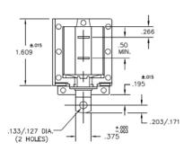
Solenoid shown energized in drawing with plunger fully seated
