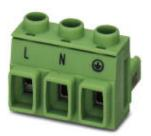
PCB connector, nominal current: 16 A, number of positions: 3, pitch: 7.62 mm, connection method: Screw connection with tension sleeve, color: green, contact surface: Tin
