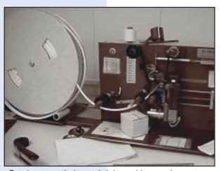
Semi-automatic heat shrink marking equipment used to provide markers for cable assemblies.
