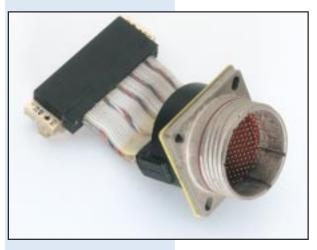
Series D38999 cable terminated to a rectangular connector for control signal termination for avionics/aircraft.
