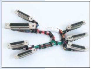
Military micro D-sub connectors, 100-pin and 50-pin, used in missile applications.
