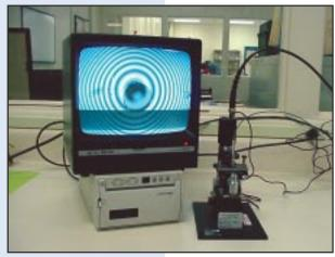
An interferometer is used for surface analysis of fiber optic cable to ensure quality.
