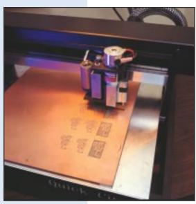
Quick circuit used for prototype and production of specialized PC boards.
