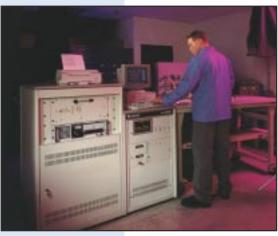
Automatic circuit analyzers (like the DIT-MCO 9500 and the Omni Tester) allow precise testing of cables, harnesses and sub-assemblies to 2,000 VDC/1,500 VAC to 2.5 Amperes. Can be configured to meet any user-specified requirement up to 100,000 test points.
