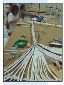
Harness assembly used in tank simulator for training.
