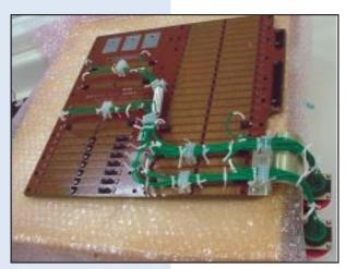
Harness composed of 25 fiber optic cable assemblies installed on a backplane for use in a missile fire control system.
