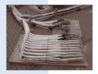
Coaxial assemblies using a Komax automatic wire cutter/stripper and terminator machine. WPI's quality assurance provides a full range of mechanical and environmental testing
