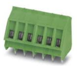
PCB terminal block, Nominal current: 24 A, Nom. voltage: 400 V, Pitch: 5.08 mm, Number of positions: 3, Connection method: Screw connection with tension sleeve, Mounting: Wave soldering, Conductor/PCB connection direction: 55 °, Color: green, The article can be aligned to create different nos. of positions!
