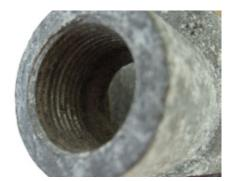
The T&B Fittings conduit bodies display clean threads with only salt deposits.
