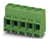
PCB terminal block, nominal current: 76 A, pitch: 10.16 mm, number of positions: 5, connection method: Screw connection with tension sleeve, mounting: Wave soldering, conductor/PCB connection direction: 0 °, color: green
