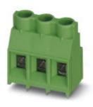
PCB terminal block, nominal current: 32 A, pitch: 7.62 mm, number of positions: 3, connection method: Screw connection with tension sleeve, mounting: Wave soldering, conductor/PCB connection direction: 0 °, color: green. The article can be aligned to create different nos. of positions!
