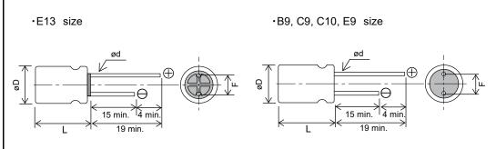
Flat rubber is used for B9, C9, C10, and E9 size.
