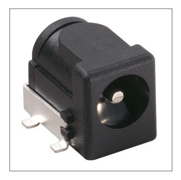
Power supply chassis socket, angular version, with break contacts, for printed circuit boards, surface mounting technology (SMT)
