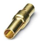
Crimp contact, turned, Single contact, contact diameter: 1 mm, crimp range: 0.08 mm<sup>2</sup> ... 0.22 mm<sup>2</sup>
