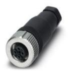
Sensor/actuator connector, female, straight, 5-pos., M12 SPEEDCON, A-coded, screw connection, metal knurl, cable screw connection Pg7
