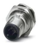
Sensor/actuator flush-type plug, 5-pos., M12 SPEEDCON, A-coded, rear/screw mounting with Pg9 thread, with straight solder connection
