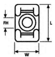
KR mounts give additional support to the cables by means of their curved design. Simple to install with a screw or bolt they give excellent security, particularly in areas of high vibration when used in conjunction with the KR straps. They must offer one of the most vibration resistant fixings available.
