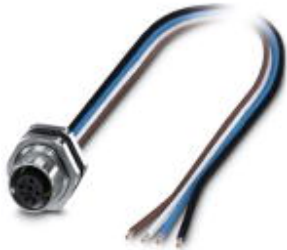
Flush-type connector, Universal, 5-position, Socket, M12, A-coded, Rear mounting, M16 x 1.5, Individual wires, cable length: 0.5 m
