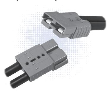
Like the other Multipole connectors, the SB®120 offers color-coded mechanically keyed housings. Keys can be used to identify and separate different circuits, or prevent users from accidentally cross mating different voltages. Wires sizes from #10 (5.3 mm²) to #1 (42.4 mm²) are held in the second smallest SB® housing.
