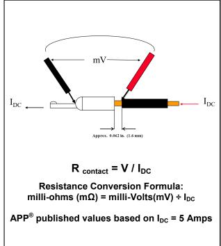
The included crimp performance and dimensional information are provided as a means to verify quality crimping of Anderson Power Products® (APP®) contacts and is based on the use of APP® tooling. The assembly of connector solutions with APP® tooling assures that all crimp performance and fit specifications are met. Customers must regularly re-check electrical performance and dimensions of crimps to determine if APP® crimp tools require maintenance due to wear over time.
