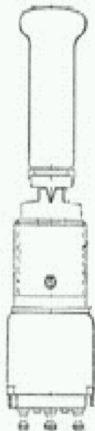
TW Series Toggle Switch, 2 pole, 2 position, Solder terminal, Locking Lever
