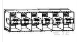
TE Model / Part #2198339-7 zSFP+ STACKED 2X6 RECEPTACLE ASSEMBLY
