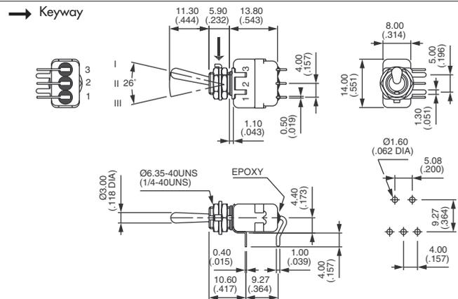
▲ Models with straight PC terminals are also available with 3,5 mm (.138) short terminals, functions 6, 9, 7 and 8. On request.
