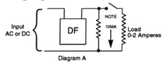
Note: Optional 10 MA load may be used to reduce initial delay time.
