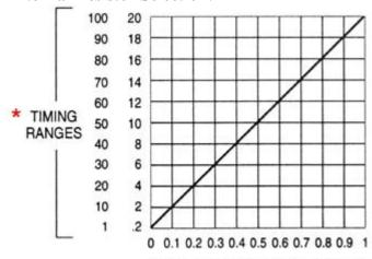
TIMING RESISTOR IN MEGOHMS
