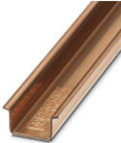
DIN rail, material: Copper, unperforated, 1.5 mm thick, height 15 mm, width 35 mm, length: 2 m
