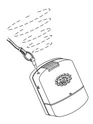
To activate both Mugger Stopper Plus alarm and strobe light, simply pull out pin on top of unit.
