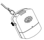
To turn on built-in flashlight, slide button up on the side of the unit.
