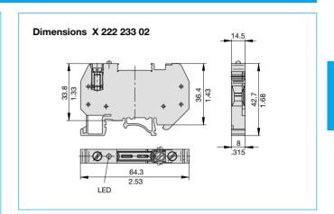
**Vibration** with terminal block X 222 233 01 and X 222 233 02  $5 g (57-500 Hz), \pm 0.38 mm (10-57 Hz)$ to IEC 60068-2-6, test Fc, 10 frequency cycles/axis and EN 50155 with terminal block X 222 233 01 Shock and X 222 233 02 25 g (11 ms) to IEC 60068-2-27, test Ea
