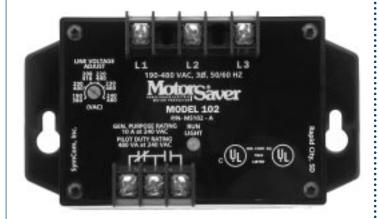
**The Model 102A** is an auto-ranging voltage monitor designed to protect 3-phase motors regardless of size. It is used on 190-480 VAC, 50 to 60 Hz motors to prevent damage caused by single phasing, low voltage, phase reversal, or voltage unbalance.
