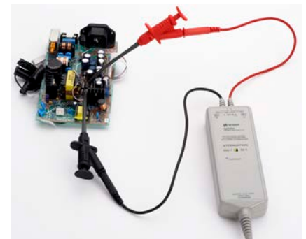
N2790A measuring a power supply signal
