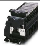
Fuse modular terminal block, without fuse plug, Connection method: Screw connection, Cross section: 0.5 mm²- 16 mm², AWG: 20 - 6, Nominal current: 10 A, Nominal voltage: 500 V, Width: 10.2 mm, Fuse type: G / 5 x 20 / 5 x 25 / 5 x 30 / 6.3 x 32, Fuse type: Glass / ceramics / ..., Mounting type: NS 35/7,5, NS 35/15, NS 32, Color: black
