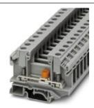
Universal terminal block with bolt connection, with test socket screws and disconnect slide, cross section: 0.1 - 6 mm², width: 11 mm, color: Gray
