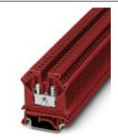
Feed-through terminal block, Connection method: Screw connection, Cross section: 0.2 mm<sup>2</sup> - 4 mm<sup>2</sup>, AWG: 24 - 12, Width: 5.2 mm, Color: red, Mounting type: NS 35/7,5, NS 35/15, NS 32
