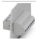
Panel feed-through terminal block, Connection method: Screw connection, Load current: 76 A, Cross section: 0.5 mm² - 16 mm², AWG 20 - 6, Connection direction of the conductor to plug-in direction: 90 °, Width: 10.1 mm, Color: gray
