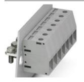
Panel feed-through terminal block, Connection method: Screw connection, Cable lug connection, Load current : 150 A, Cross section: 16 mm<sup>2</sup> - 50 mm<sup>2</sup>, AWG 6 - 1/0, Connection direction of the conductor to plug-in direction: 0 °, Width: 18.8 mm, Color: gray
