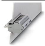
Panel feed-through terminal block, Connection method: Screw connection, Solder/Slip-on connection, Load current: 18 A, Cross section: 0.2 mm² - 6 mm², AWG 24 - 10, Connection direction of the conductor to plug-in direction: 0 °, Width: 6.2 mm, Color: gray
