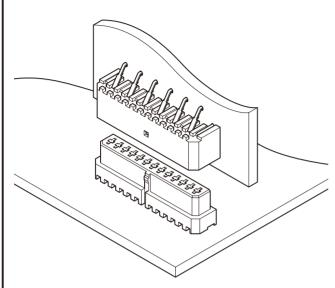
The JE connector is a compact, board-toboard connector only 6.8mm high and 3.6mm wide. Its mating part has a 1.25mm pitch, single row construction. High contact pressure dual beam fork contacts are combined with a housing lock mechanism to ensure a reliable connection.
