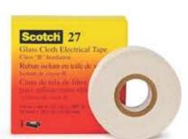
Ideal for electrical maintenance applications, this is a 7 mil woven glass cloth tape with a rubber thermosetting pressure-sensitive adhesive. UL Recognized 130(deg)C. Printable. Sold on a 1 inch paper core with an inner pack of 1/box with 10/carton.
