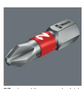
BiTorsion bits are absolutely premium products. They have a softer BiTorsion zone which reduces the hardness of the shaft by about 20 % in comparison to the drive tip. This means that the peak loads that cause bit breakage and premature wear are absorbed in this zone — something which enhances the service life of the bits.
