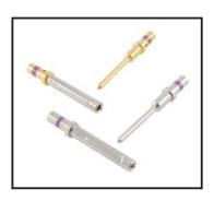
The new size 20 contacts provide versatility within the Deutsch common contact system. The contacts feature a size 20 mating interface and a 16-18 AWG crimp barrel to accept larger wire while mating with any Deutsch Industrial size 20 contact.
