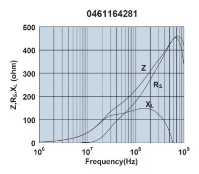
Impedance, reactance, and resistance vs. frequency.
