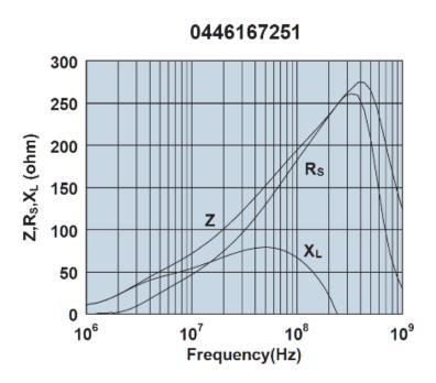
Impedance, reactance, and resistance vs. frequency.
