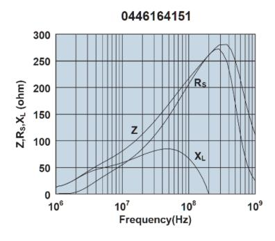
Impedance, reactance, and resistance vs. frequency.
