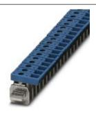
Connection terminal block, connection method: Screw connection, load current: 41 A, cross section: 0.5 mm² - 6 mm², width: 7 mm, color: blue
