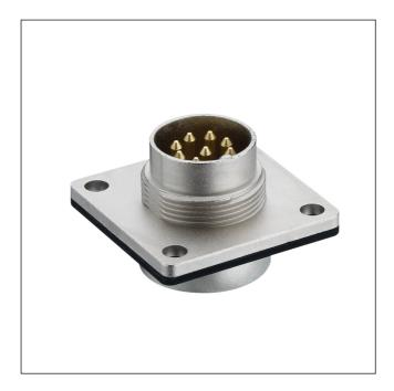
SWUM<sup>™</sup> flange chassis plug acc. to IEC 61076-2-106 and AISG specification, IP68/67, with threaded joint and solder terminals, for front mounting
