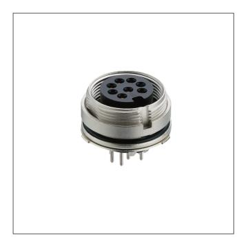
SWUM<sup>™</sup> chassis socket acc. to IEC 61076-2-106 and AISG specification, IP68/67, with threaded joint and ground contact, for printed circuit boards, manual soldering, for back side mounting
