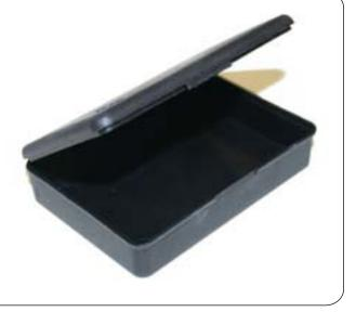
These boxes are made of conductive polypropylene with a surface resistivity of approximately  $5 \times 10^3$  ohm per square and a volume resistivity of about  $10^4$  ohm cm providing an excellent shield against electrostatic fields as defined in IEC 61340-5. They are suitable for primary packaging of electrostatic sensitive devices that do not have a built-in power source.
