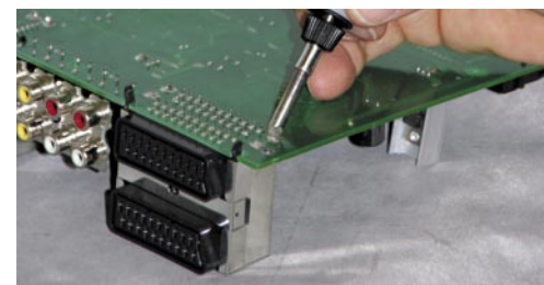
High mass Through hole soldering.
